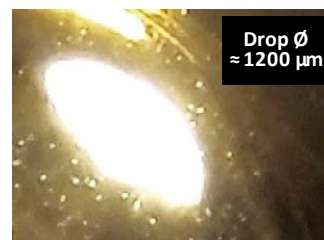
Fig. 2 : → Movie 2 : Evaporation of a water droplet on a gold surface. The movie shows how the water drop finally shrinks (evaporates) around a larger cluster, that probably is a particle of the small amount of washing powder which I added to the distilled (clean) water.
