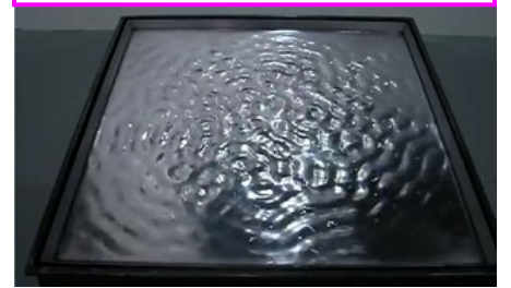
Movie_7 : Water excited with A=440 Hz & A=432Hz Sine, Square & Sawtooth Waves
