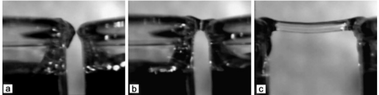
Figure 1. Water bridge formation: (a) Rise of water in both beakers after a high voltage was applied and a first ignition spark was observed , (b) spontaneous formation of a connection which remains stable after (c) pulling the beakers apart .
